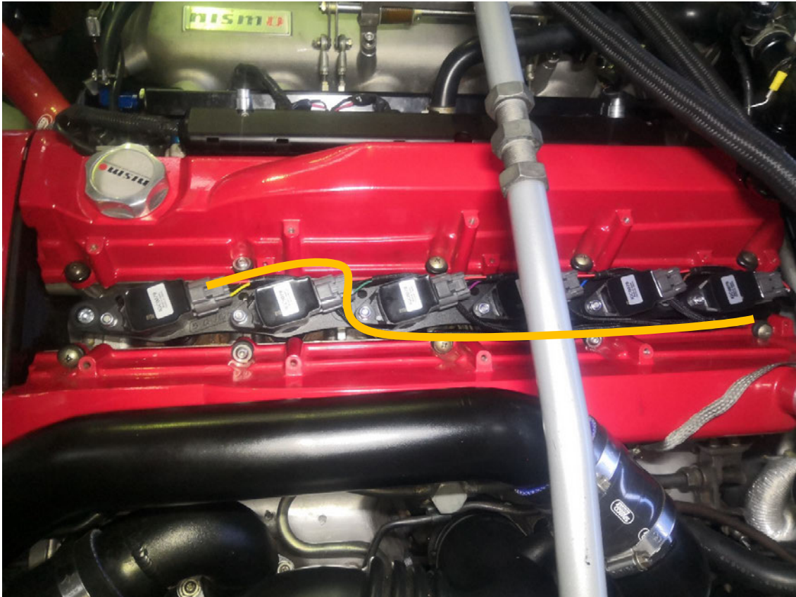
Figure 4 – Install the Coil Kit and Harness to the Engine (All RB except RB25 NEO)
