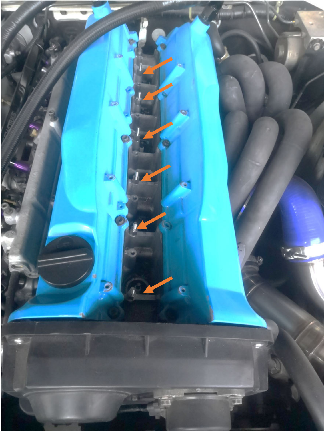
Figure 5 – M6 Standoff Position for RB25 NEO
