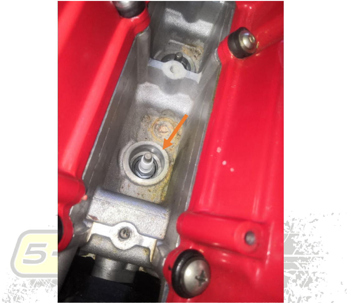
Figure 2 – Clean the Top Surface of the Spark Plug Bore
