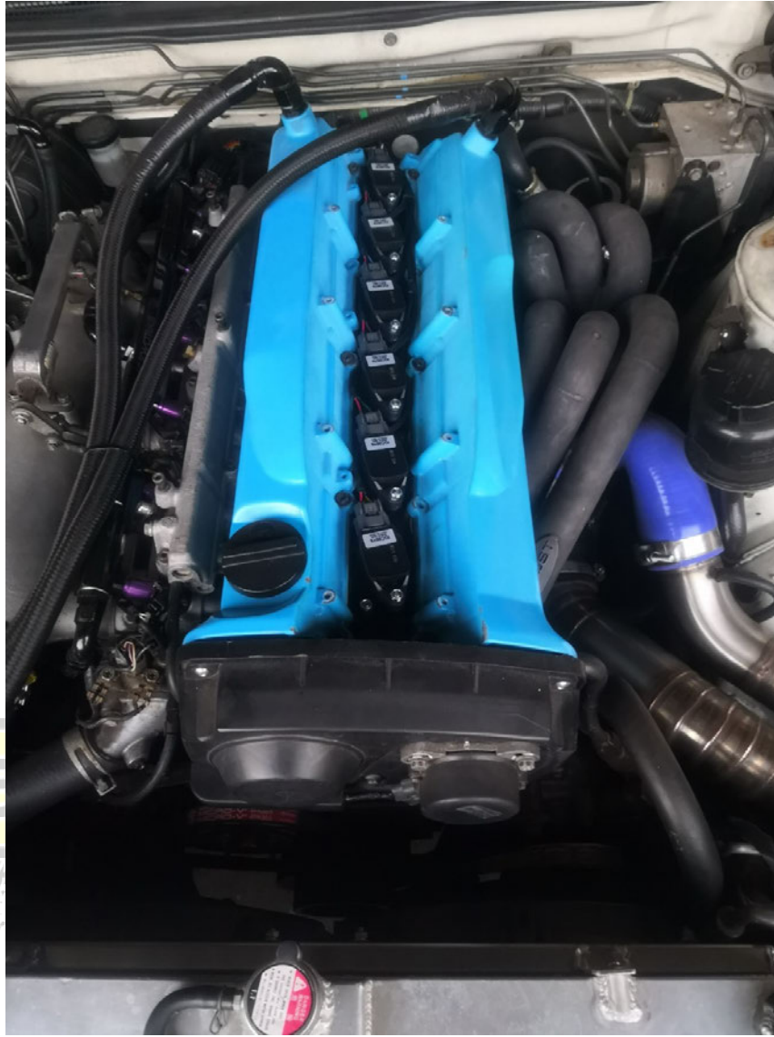
Figure 6 – Install the Coil Kit and Harness to the Engine (RB25 NEO Only)
