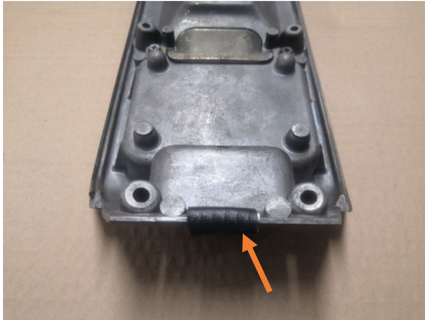
Figure 9 – Install the Supplied Pinch Weld Grommet to Protect Wiring Harness from Abrasion (RB26DETT Only)
